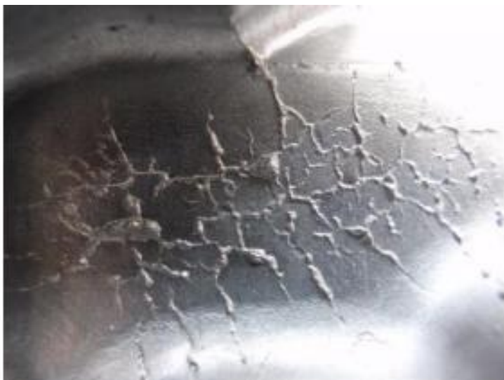
Thermal shock on a die causes cracking
