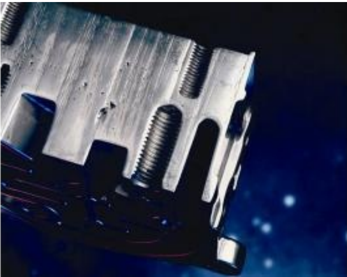
Component with Porosity
